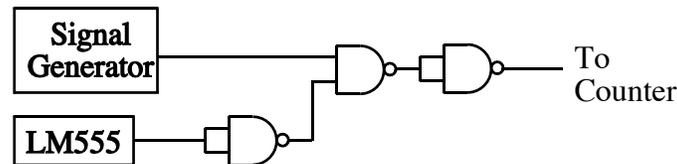
Figure 7s.2 Counter Input Gating using NAND gates
