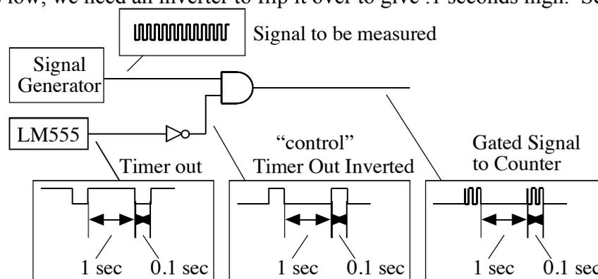
Figure 7s.1 The Counter Input Gating
