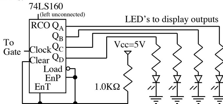
Figure 7s.3 Decimal Counter Circuit
