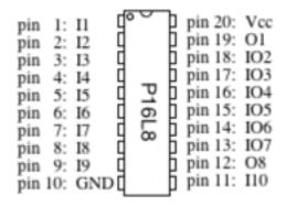
Power connections are at the corners, similar to most TTL chips. Pins labeled I1 to I10 can be used for inputs. Those labeled O1 and O8 can only be used for outputs. Those labeled IO2 to IO7 can be used as either inputs or outputs (or both, if you don't mind an output being connected back to an input).
