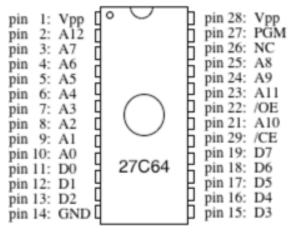
Power: Connect Vcc and Vpp to 5 Volts. (Pin 27 is grounded for the 27256.) (The programmer will put a higher voltage on Vpp during programming, but you don't have to worry about that.) Connect GND to your ground. Also, connect "Chip Enable" (active low) and "Output Enable" (also active low) to Ground; we will leave the device on all of the time. In computers, /CE and /OE are used to control when the device is being read and when it is not.
