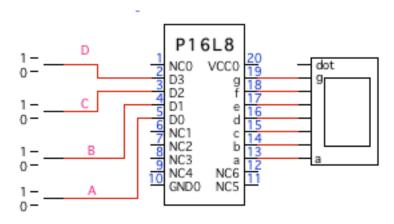
This figure shows the use of a ".dwl file" in Logicworks to simulate with the part.
